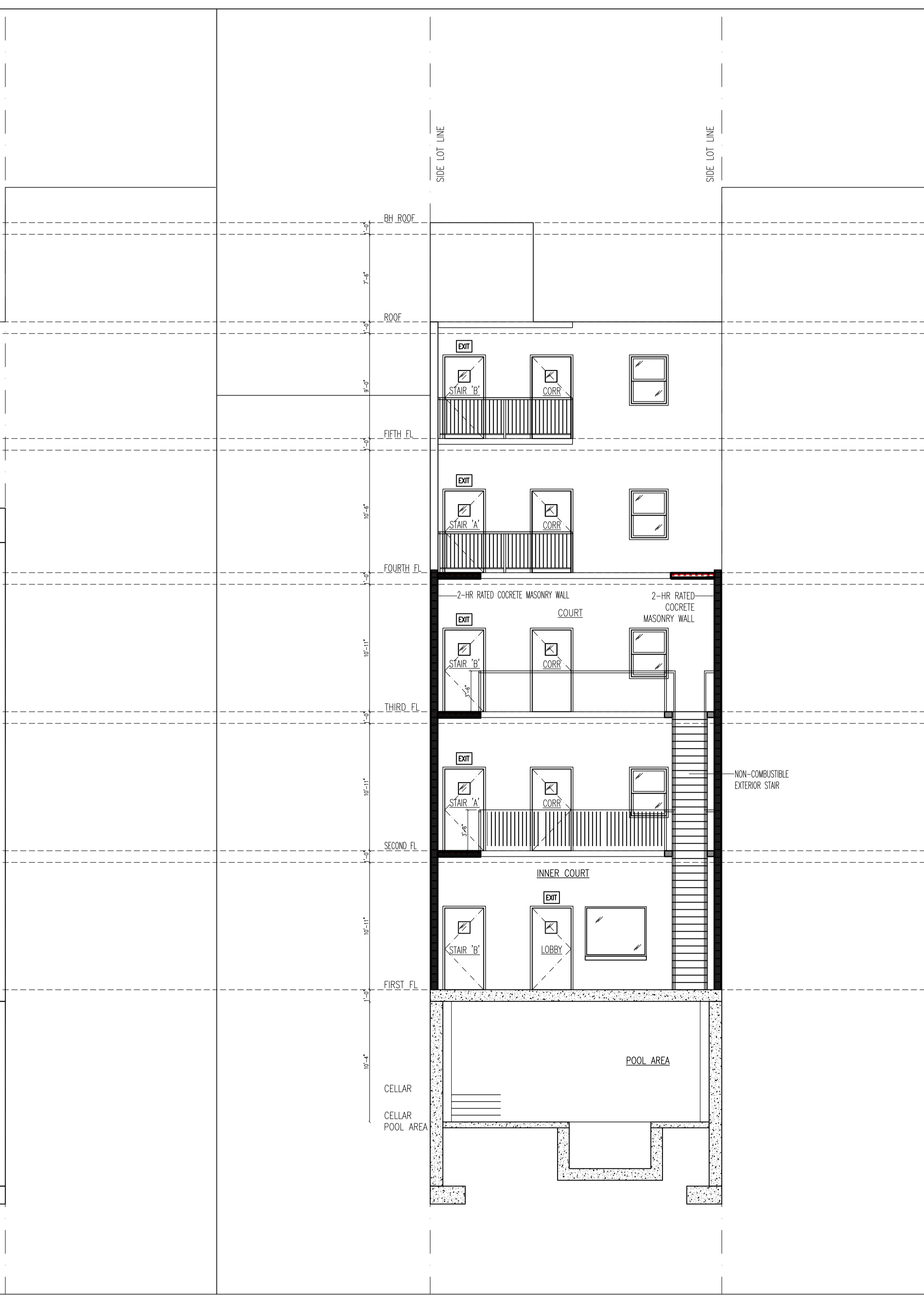
2 Transverse Section 2 (Through Courtyard) SCALE: 3/16" = 1'-0"
